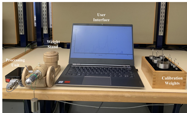
Fig. 5. Wireless pelvic floor muscle measurement system experimental setup.
